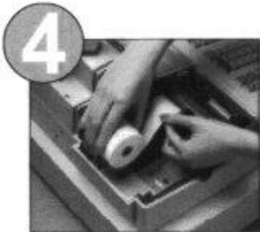
5. Pass the paper over the black roller and insert the end into the space behind the printer
